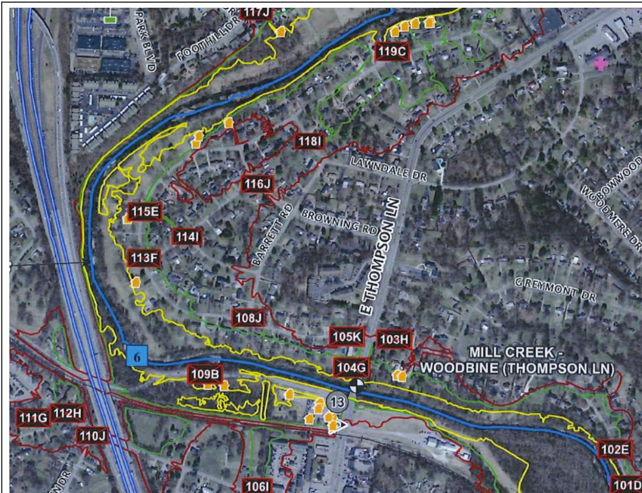
Inundation maps for Action Levels B, F and K at the Mill Creek gauge near Woodbine.
