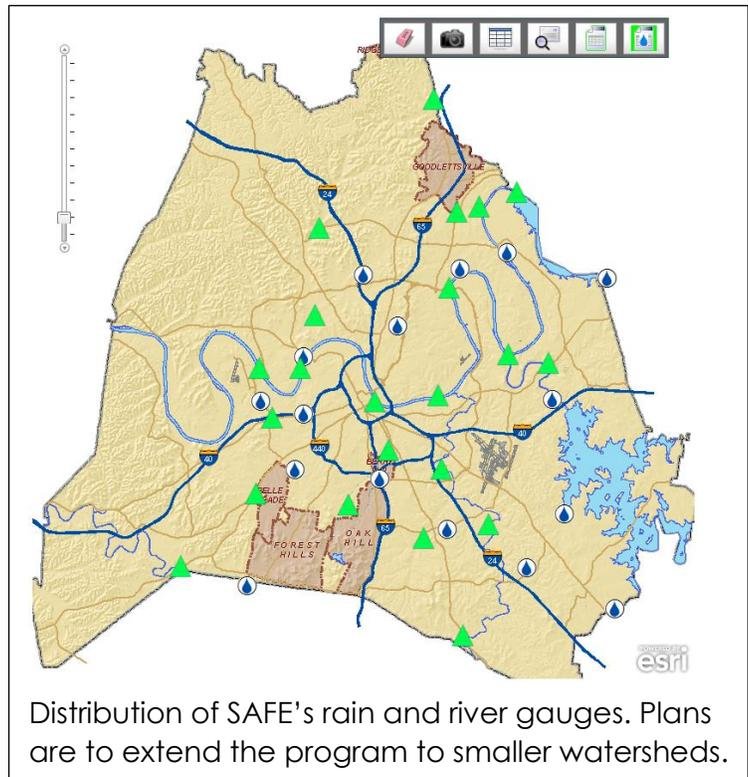
Distribution of SAFE's rain and river gauges. Plans are to extend the program to smaller watersheds.
